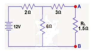
21. Find the value of  $R_L$  for maximum power in the circuit of fig given below. Also find the maximum power.
